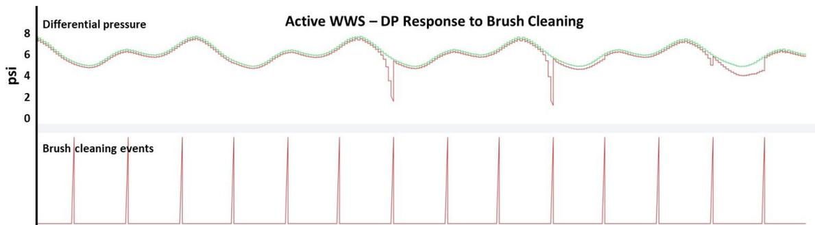
Figure 19. Effectiveness of cleaning method for controlling DP in pilot-scale active wedgewire intake screening assembly. Data show a four-day period (December 29, 2020 – January 2, 2021) during which a suspected clogging event occurred.
