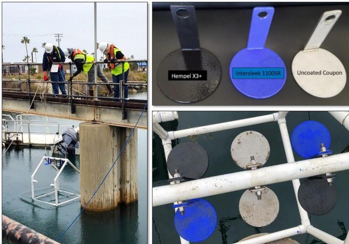
**Figure 11. PVC frame for deploying coupons (left), coupons prior to deployment (top right), and coupons after two weeks of immersion (bottom right).**
