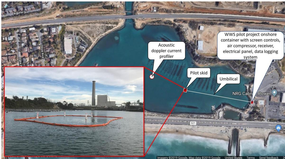
**Figure 1. Generalized site plan for the WWS Pilot Project showing the offshore and onshore components; inset is a photo of the boom and warning buoys installed to mark the stand-off zone around the submerged skid.**
