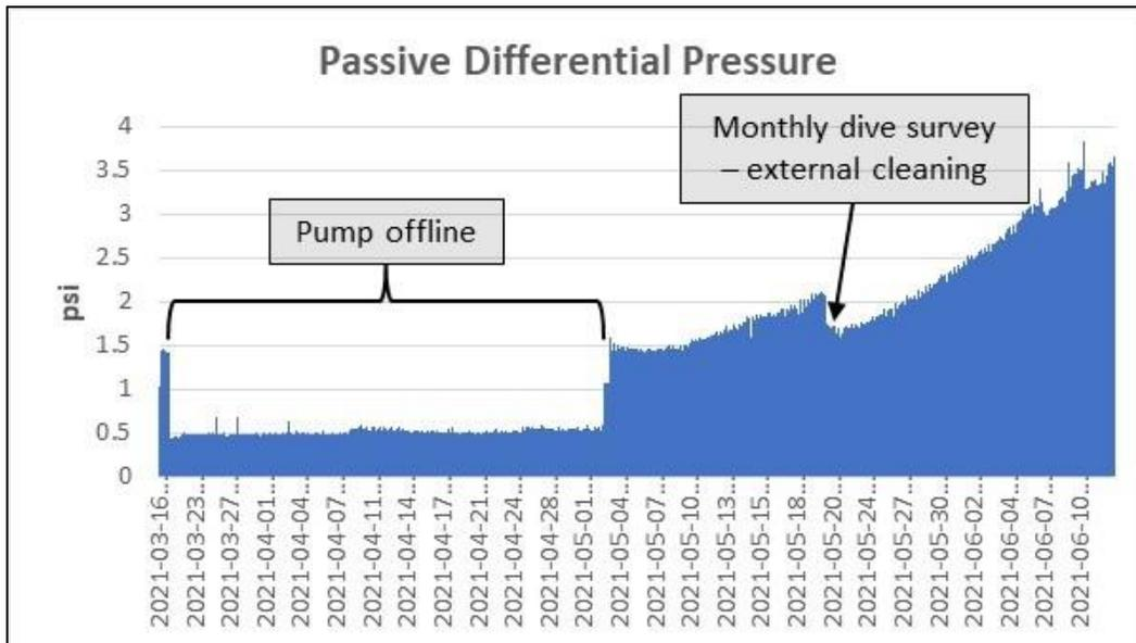
Figure 21. Differential pressure through passive wedgewire screening assembly during Q2.
