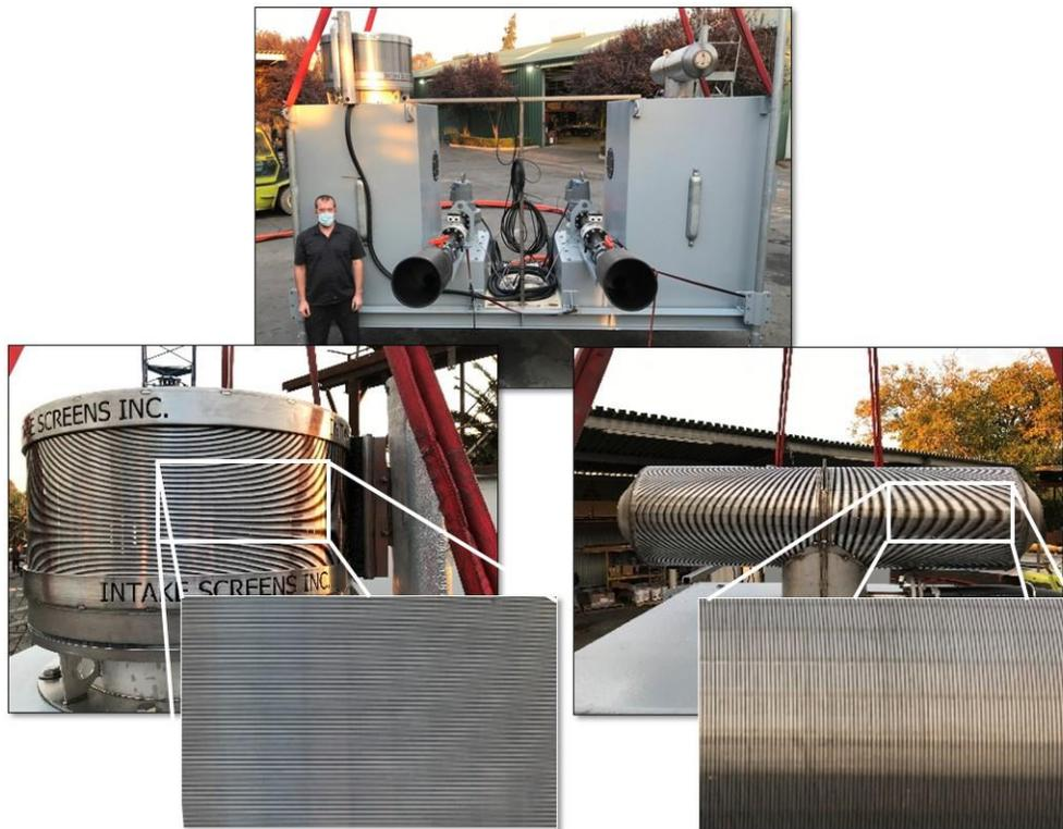
**Figure A-1. WWS Pilot Project skid (top), pilot-scale 1-mm active wedgewire screen from Intake Screens, Inc. (bottom left) and pilot-scale 1-mm passive wedgewire screen from Aqseptence (bottom right).**
