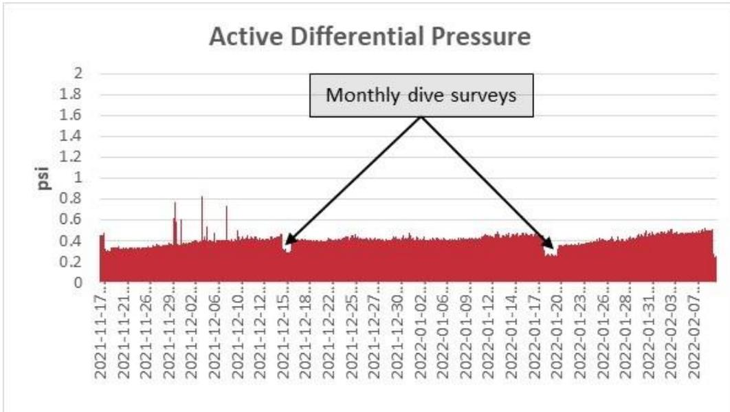
Figure 32. Differential pressure through active wedgewire screening assembly during Q4.
