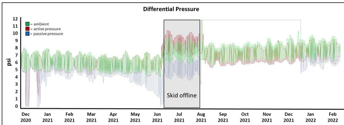
**Figure 13. Unplanned offline period (associated with the skid becoming partially un-anchored) based on differential pressure. Note the passive WWS decrease in pressure (i.e., increase in differential pressure) between mid-April and mid-June 2021. At the time the skid becomes partially un-anchored (gray box), the active and passive pressure transducers shift depth as well – captured as the change in pressures (relative to ambient) during the offline period.**
