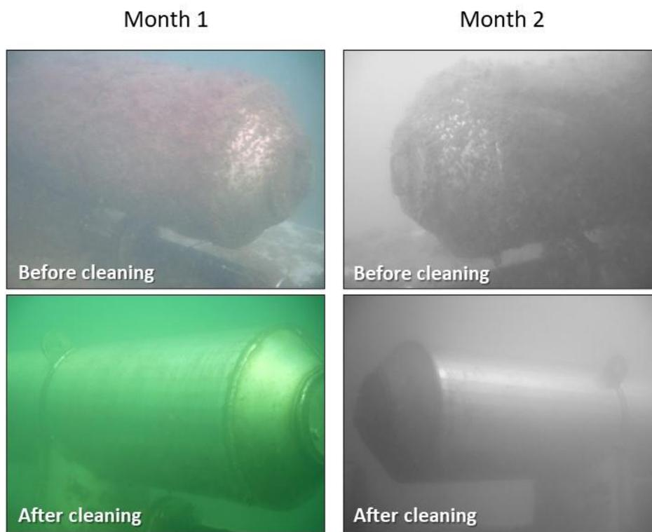
**Figure 17. Photos of the passive WWS before and after external cleaning by divers during months 1 (January 2021 dive survey) and 2 (February 2021 dive survey) of Q1. Note that no photos are available from Month 3 due to poor visibility.**
