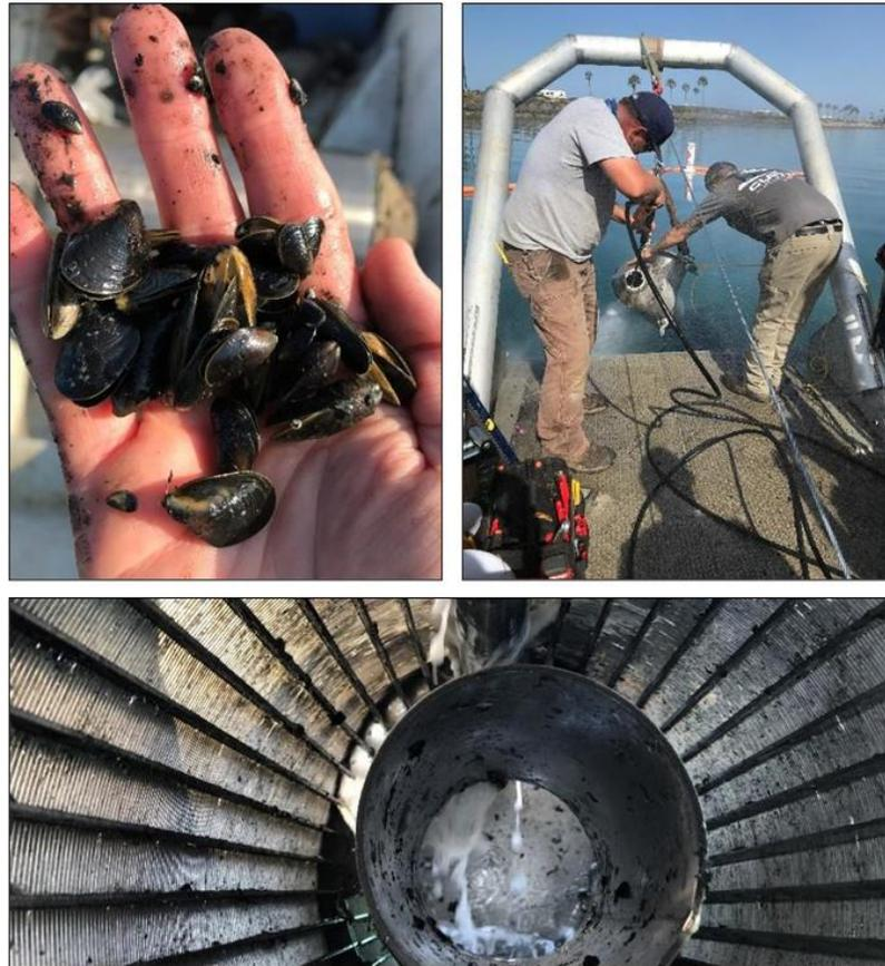
**Figure D-6. Blue mussels removed from inside passive screen (top left), divers cleaning passive screen with pressure washer after it had been recovered to the surface (top right), and view through endcap of cleaned internal surfaces.**
