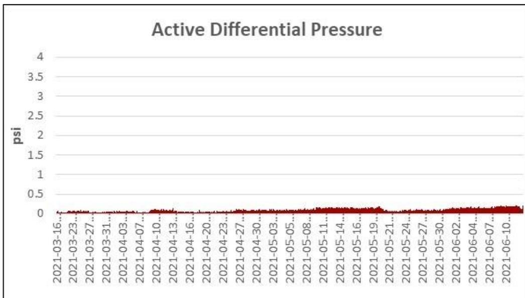
**Figure 24. Differential pressure through active wedgewire screening assembly during Q2. Note Y axis scale extends to 4 psi for comparison with the passive wedgewire screening assembly.**
