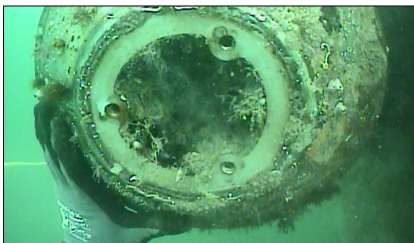
**Figure 23. Photo of biofouling inside of passive WWS after month 6 of operation (June 2021 dive survey) – endcap removed.**
