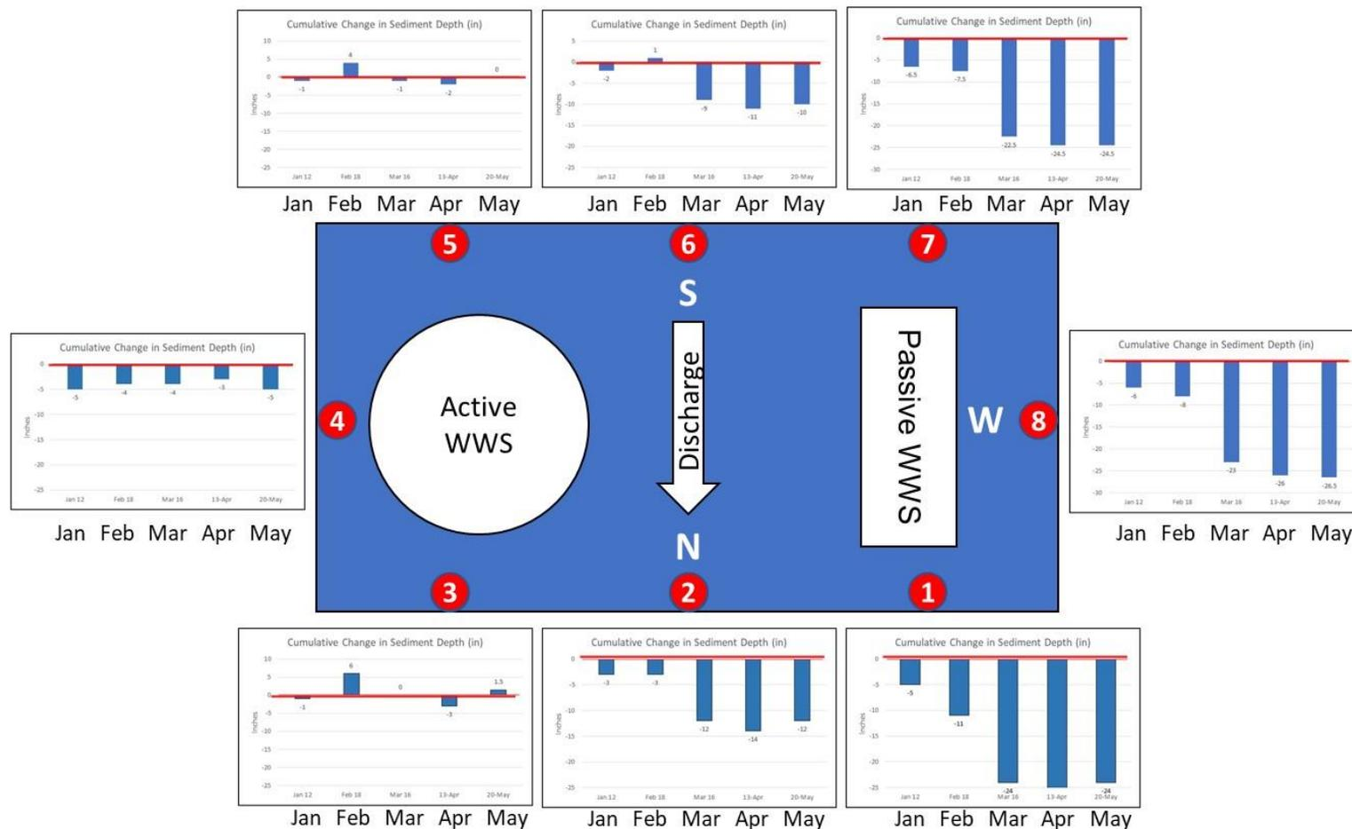
**Figure 14. Cumulative depth (inches) change by month through May 20 dive survey (Q1 and most of Q2). Change is relative to the red lines in the charts which indicate the starting depth of sediment (Dec 9, 2020): above the red line was assumed to be sedimentation; below the red line was assumed to be scour.**
