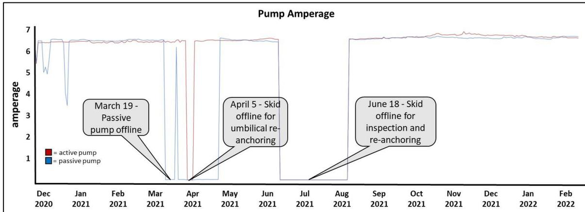
**Figure 12. Principal unplanned offline periods for the wedgewire Pilot Project based on pump amperage (on/off).**
