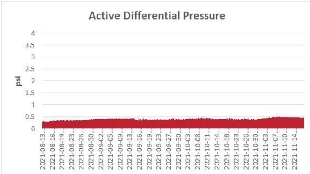
**Figure 27. Differential pressure through active wedgewire screening assembly during Q3. Note Y axis scale extends to 4 psi.**
