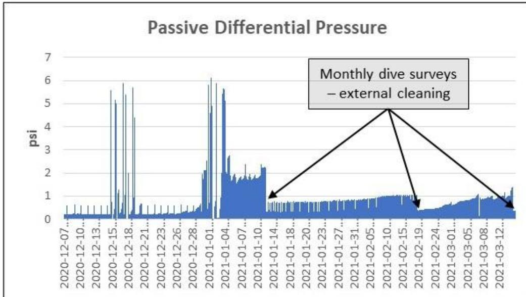
Figure 15. Differential pressure through passive wedgewire screening assembly during Q1.
