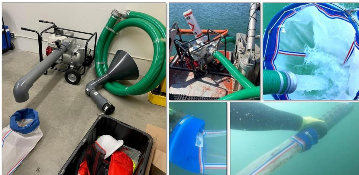
**Figure A-3. Plankton sampling gear. Clockwise from left: ambient sample collection gear (intake cone, flexible hose, trash pump, and plankton net), ambient sample collection gear in field, ambient sample discharge into plankton net, cod end of plankton net attached to discharge from a WWS, mouth of plankton net hose-clamped to discharge from a WWS**
