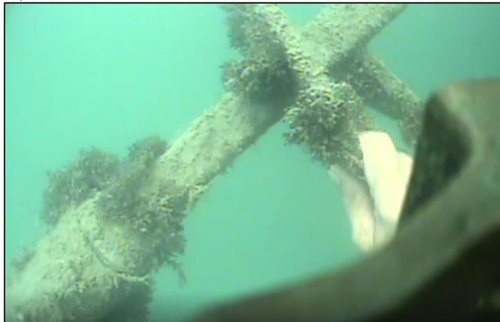
**Figure D-3. One of the two passive side helical anchors that had removed itself from the Lagoon floor during the skid tipping.**
