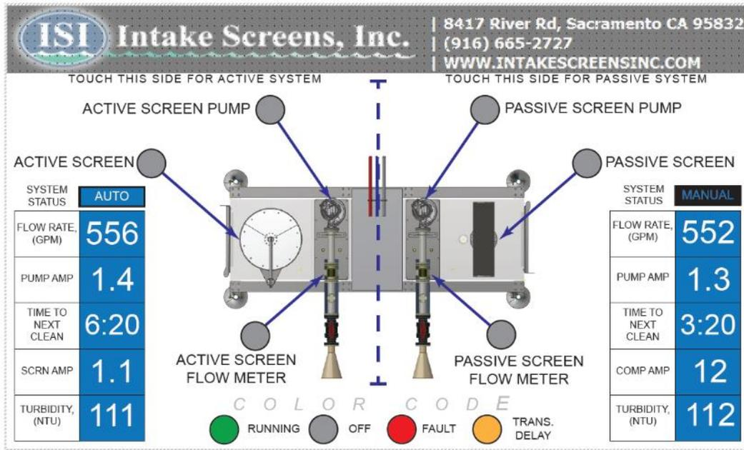
Figure 7. Example screen of the human-machine interface of the programmable logic controller.
