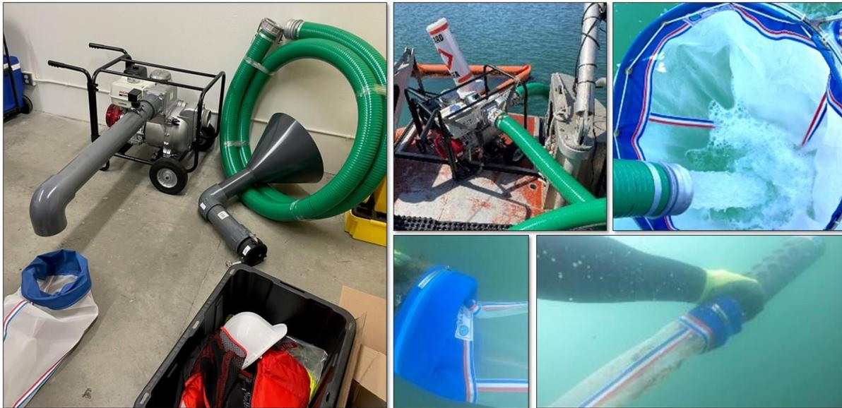
**Figure 10. Plankton sampling gear. Clockwise from left: ambient sample collection gear (intake cone, flexible hose, trash pump, and plankton net), ambient sample collection gear in field, ambient sample discharge into plankton net, cod end of plankton net attached to discharge from a WWS, mouth of plankton net hose-clamped to discharge from a WWS.**
