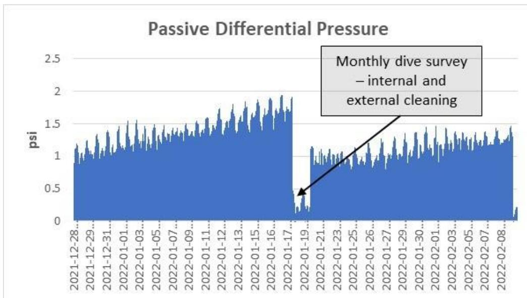
**Figure 30. Differential pressure through passive wedgewire screening assembly during Q4. Data were limited to the period after the new passive pressure transducer was installed and functioning correctly.**
