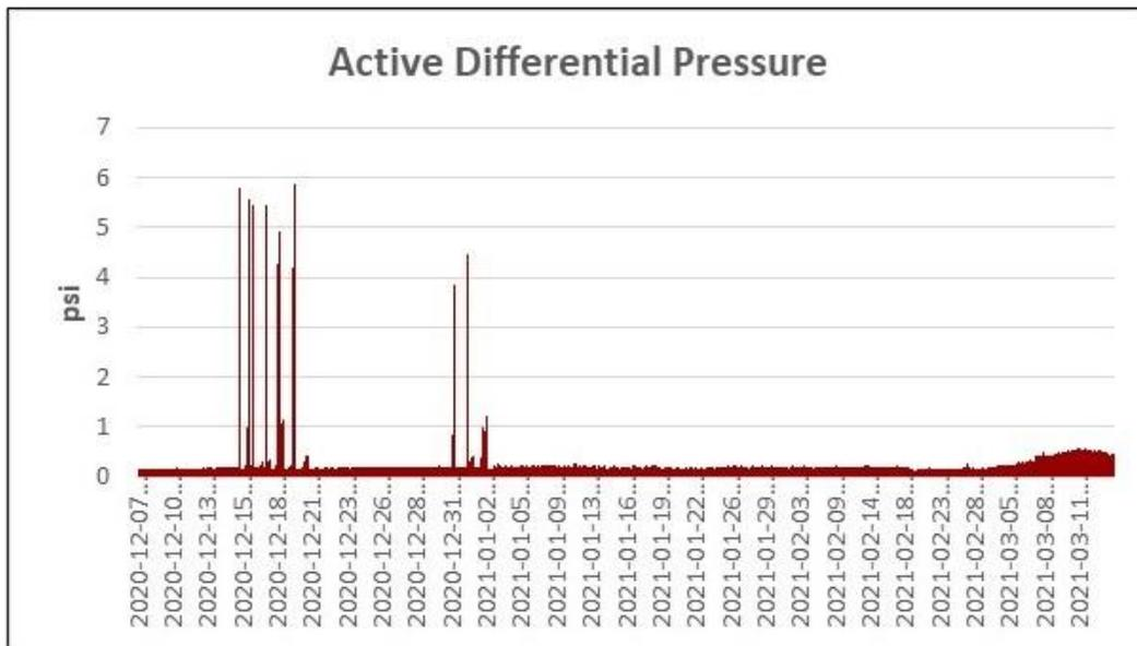
Figure 18. Differential pressure through active wedgewire screening assembly during Q1.
