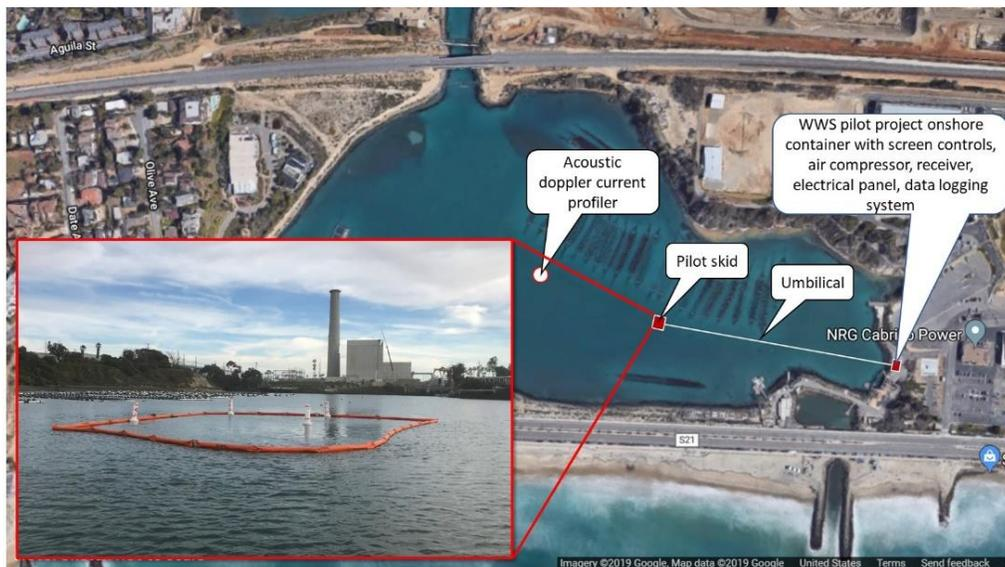
**Figure A-2. Location of the Pilot Project components. Plankton sampling was conducted at the location of the “pilot skid”. The inset photo shows the boom and warning buoys installed to mark the stand-off zone around the submerged skid.**
