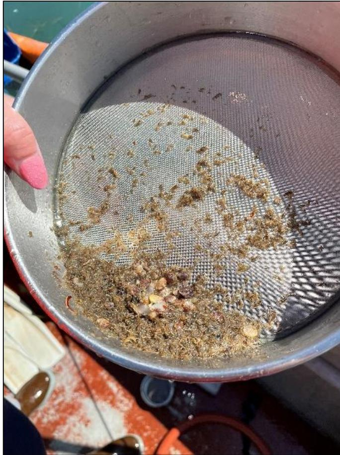
**Figure A-4. Contents from a sampling event rinsed into a 200- $\mu$ m mesh screen to condense the sample before transferring to a sample jar for later laboratory analysis.**
