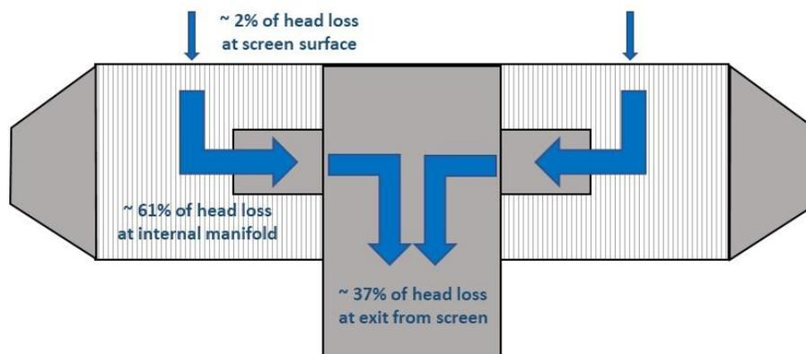
**Figure 9. Distribution of head loss through a passive WWS designed for a through-slot velocity of 0.5 ft/sec.**
