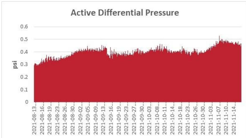
**Figure 28. Differential pressure through active wedgewire screening assembly during Q3. Note Y axis scale has been reduced substantially to illustrate a trend of increasing (albeit small) DP.**
