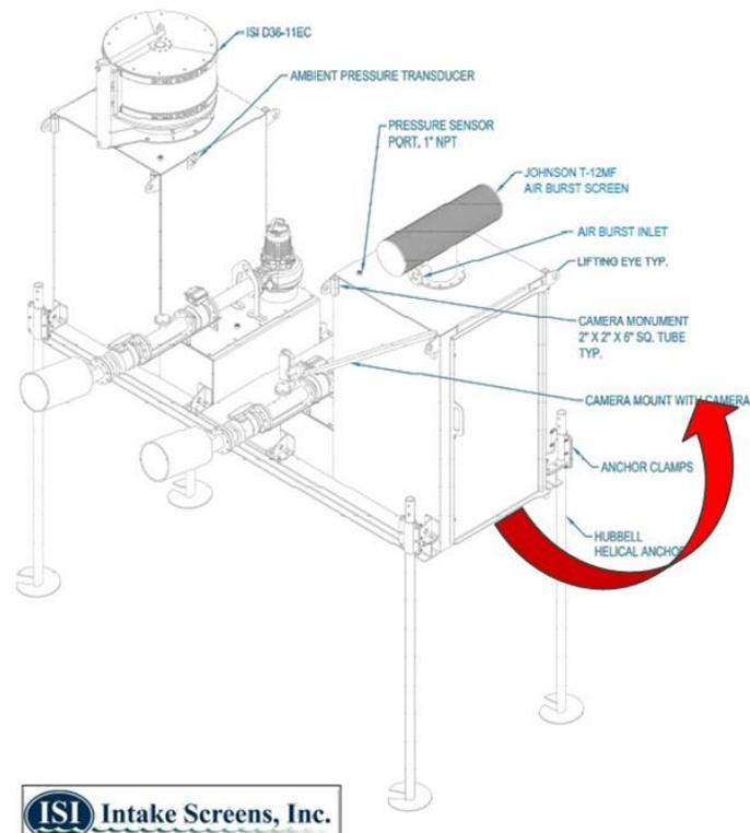
**Figure D-1. Direction that skid tipped indicated with arrow. Passive (west) side floated to surface and active (east) side sank toward Lagoon floor.**
