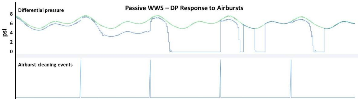
Figure 16. Effectiveness of cleaning method for controlling DP in pilot-scale passive wedgewire intake screening assembly. Data show a four-day period (December 29, 2020 – January 2, 2021) during which a suspected clogging event occurred.
