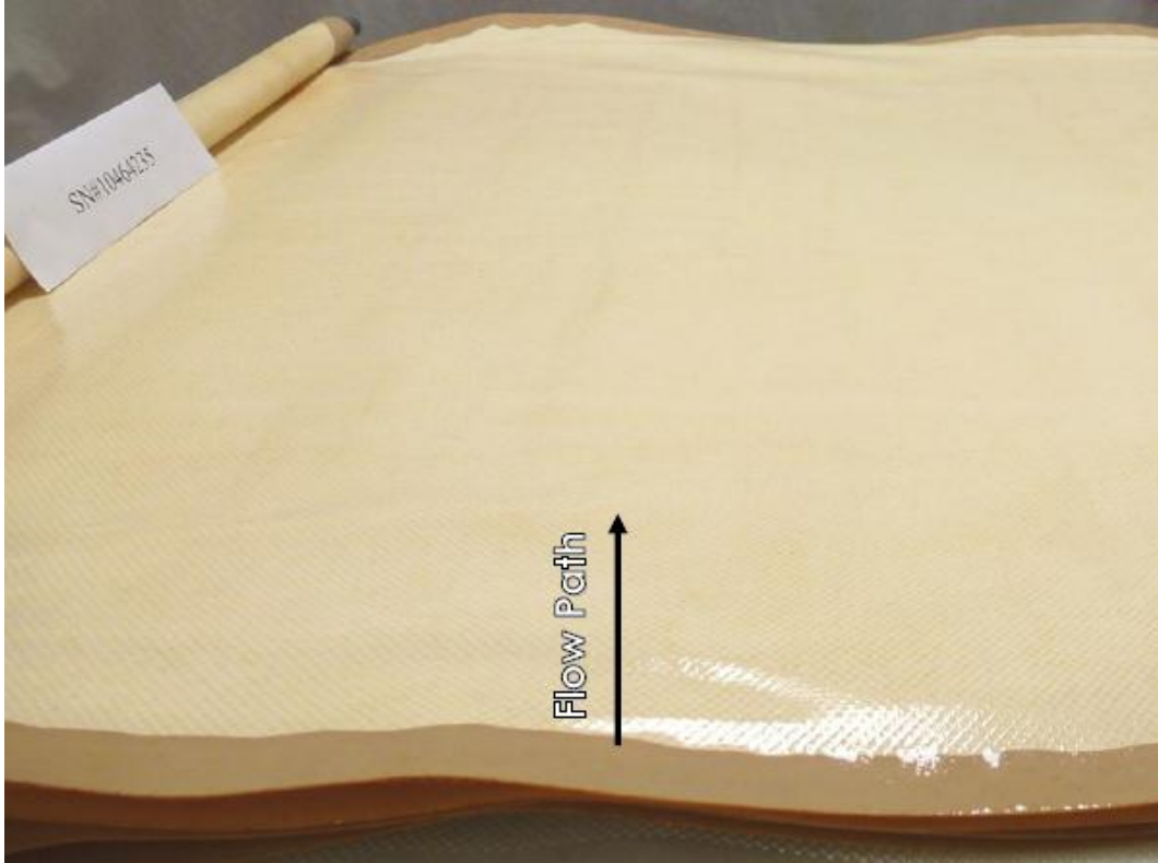
Figure 18. Photograph of the membrane surface of the tail RO element from the MBR-RO system.
