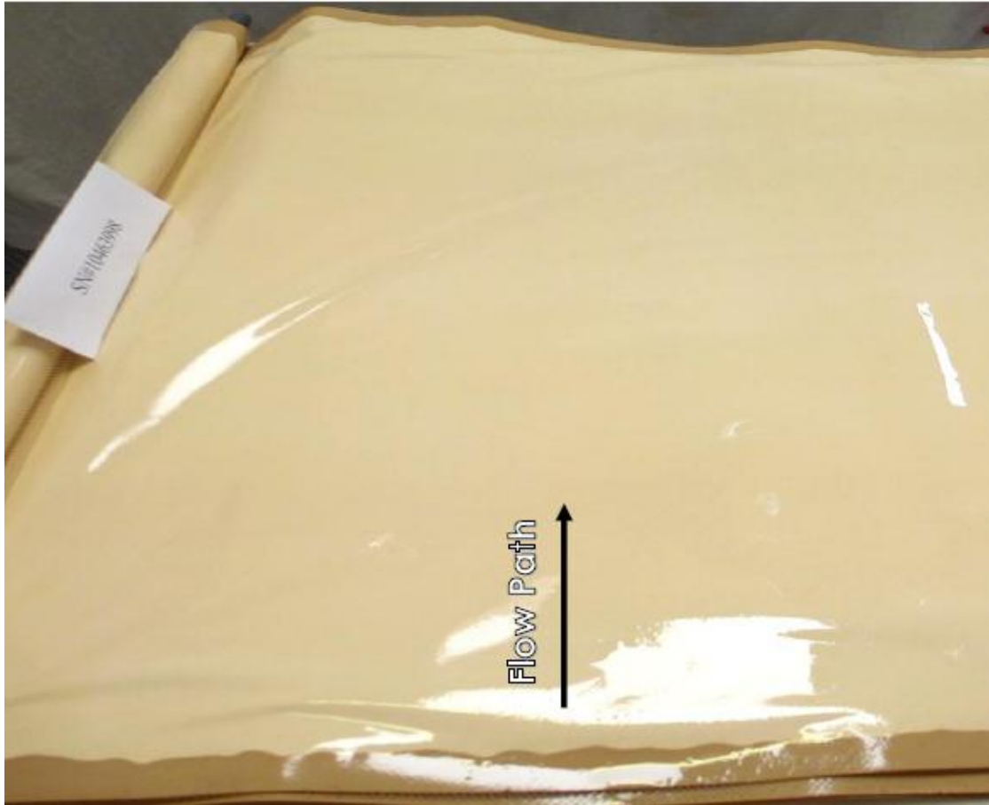
Figure 10. Photograph of the membrane surface of the tail RO element from the UF-RO system.
