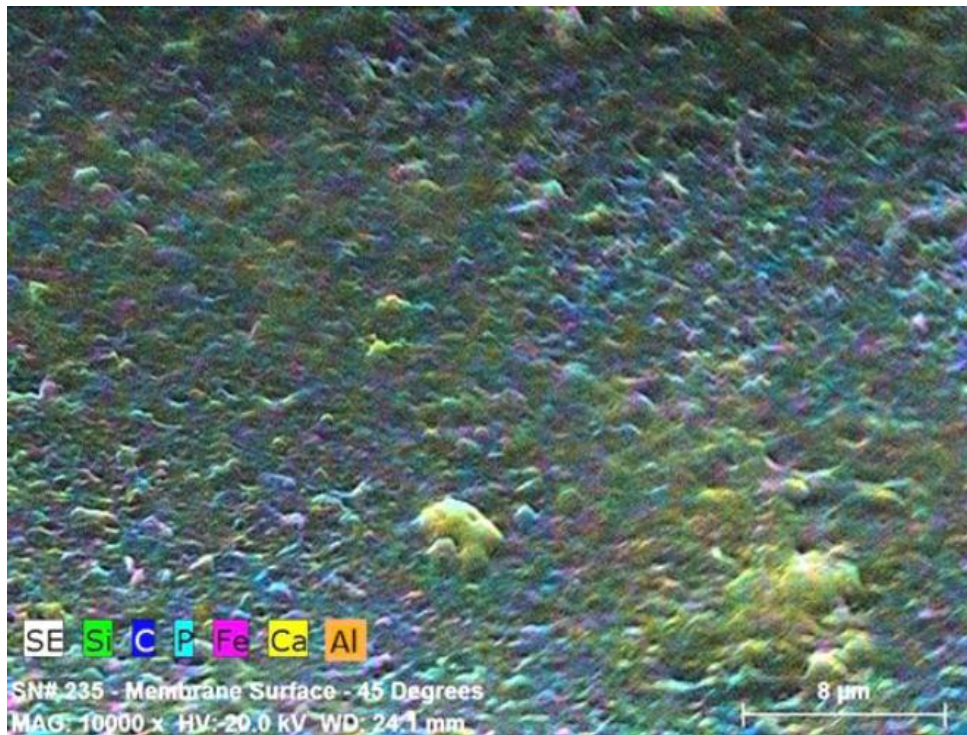
Figure 33. CEI image of membrane surface from the tail RO element membrane samples of the MBR-RO system.
