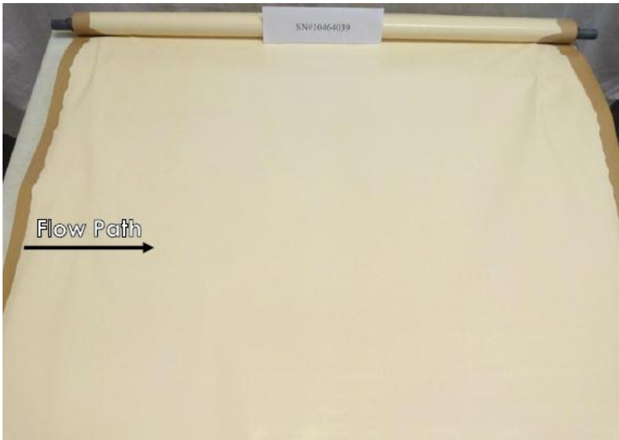
Figure 5. Photograph of the membrane surface of the lead RO element from the UF-RO system.
