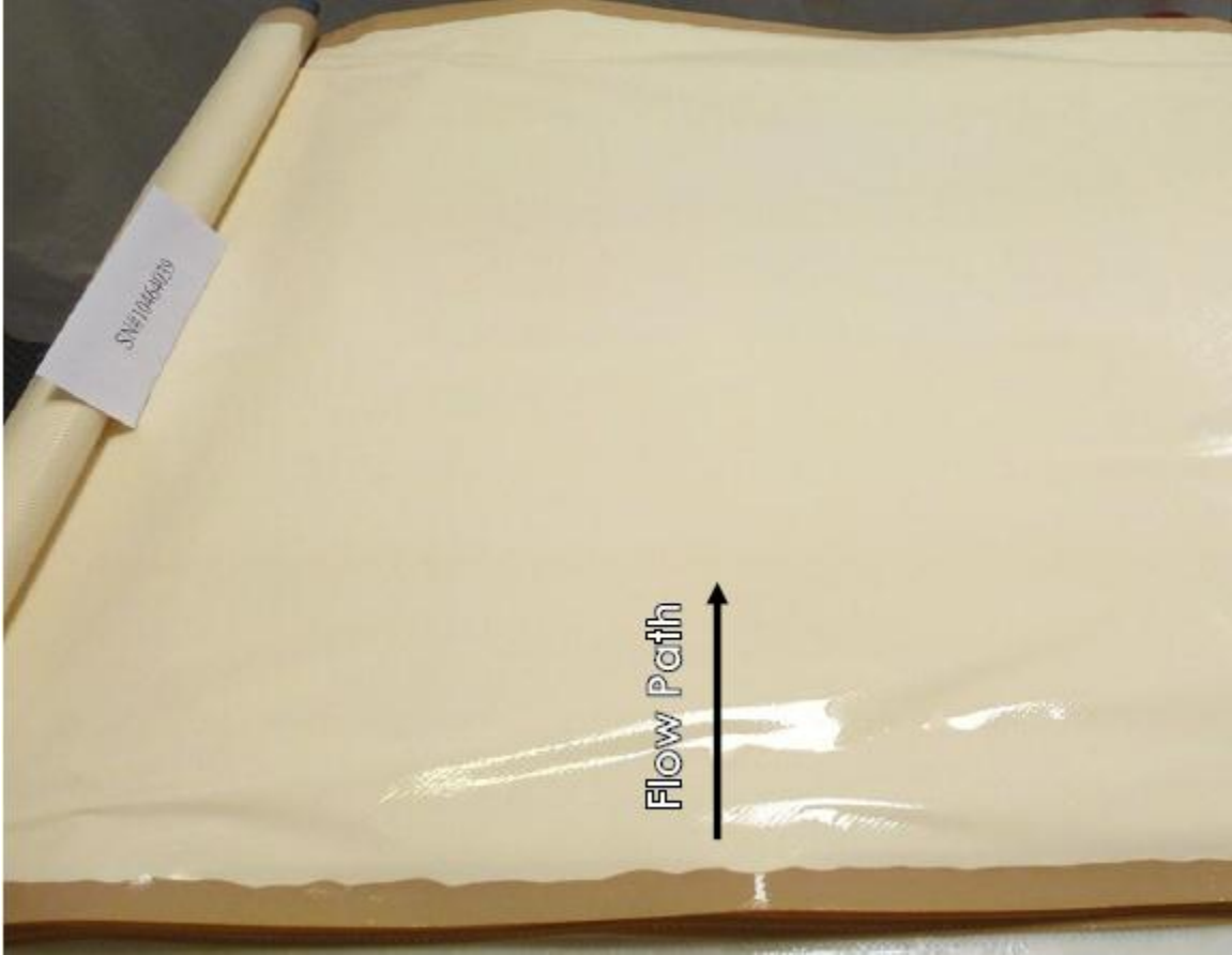
Figure 6. Photograph of the membrane surface of the lead RO element from the UF-RO system.
