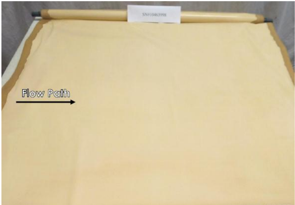
Figure 9. Photograph of the membrane surface of the tail RO element from the UF-RO system.
