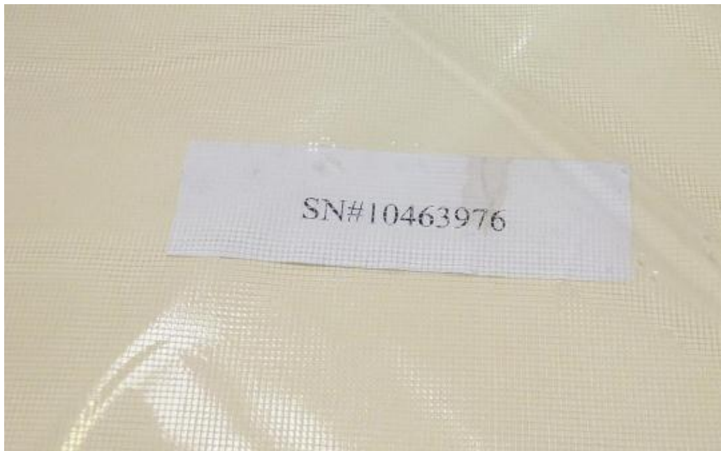
Figure 15. Image of the feed spacer of the lead RO element from the MBR-RO system.
