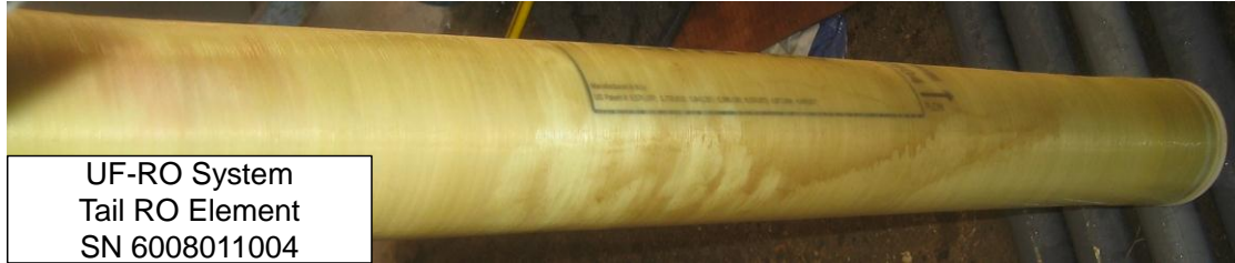
Figure 2. Photograph (taken on site) of the tail RO element from the UF-RO system.
