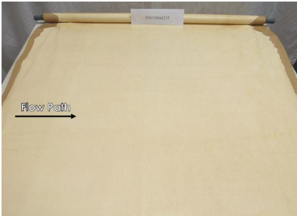
Figure 17. Photograph of the membrane surface of the tail RO element from the MBR-RO system.
