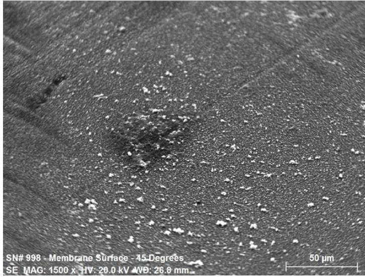
Figure 27. SEM image and EDS microanalysis of membrane surface from the tail RO element membrane samples of the UF-RO system.
