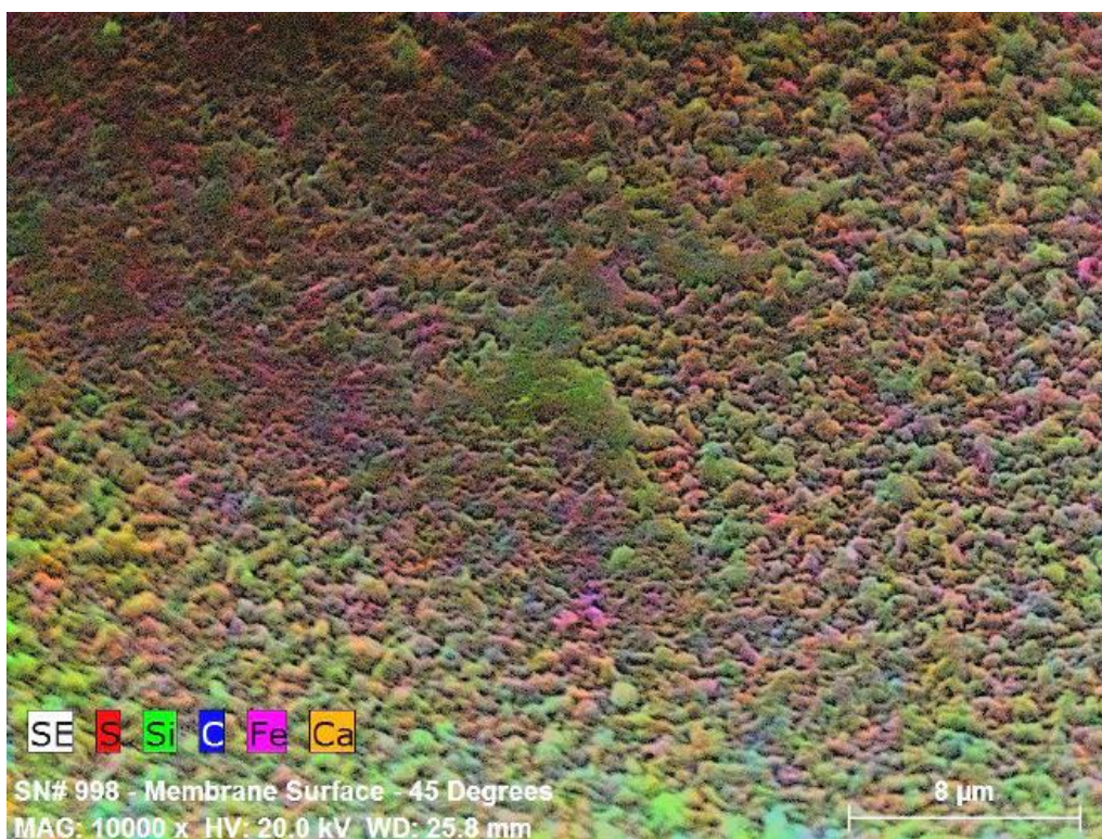
Figure 31. CEI image of membrane surface from the tail RO element membrane samples of the UF-RO system.
