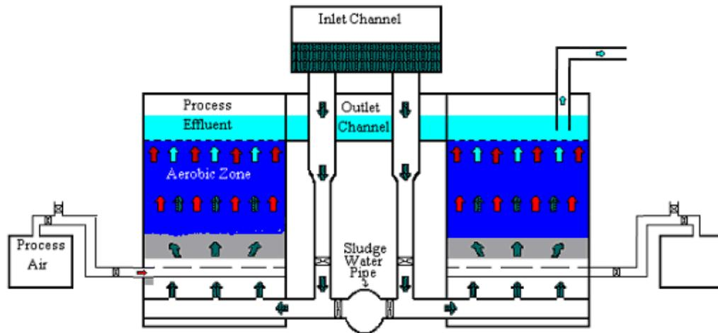
Figure 4.5 – Schematic of BIOSTYR® Process (Courtesy of Veolia)
