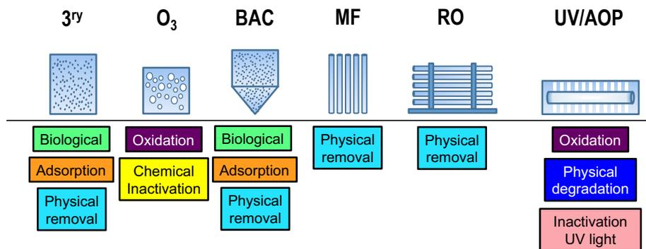
Figure 5. Multiple types of barriers provide a high degree of robustness in a DPR treatment train
