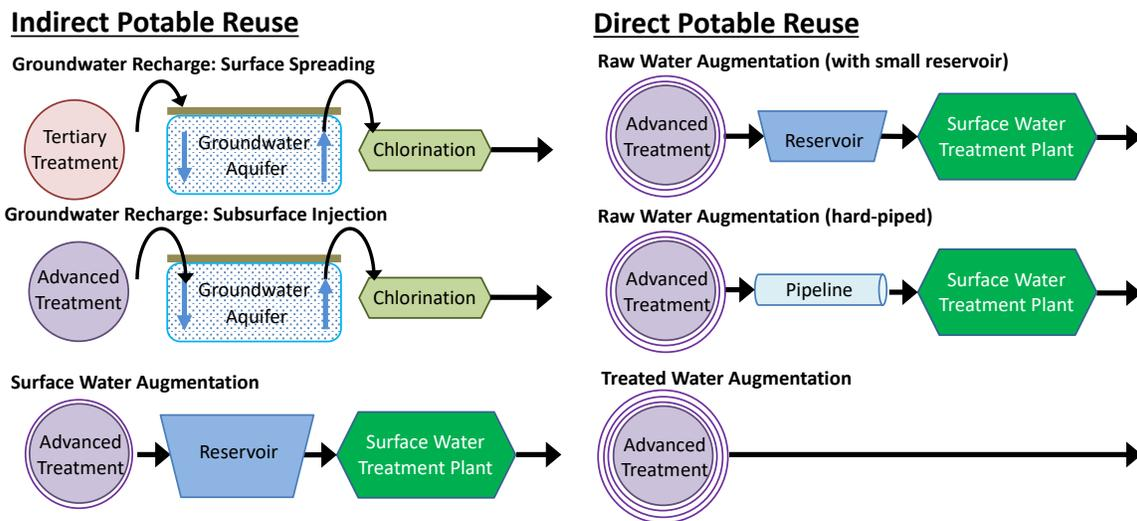
Figure 1. The six existing and anticipated forms of potable reuse in California.
