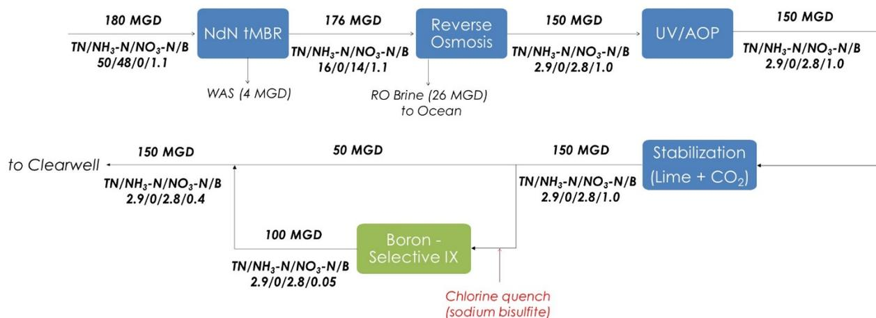
**Figure 1 – Boron-selective IX Process Train**
