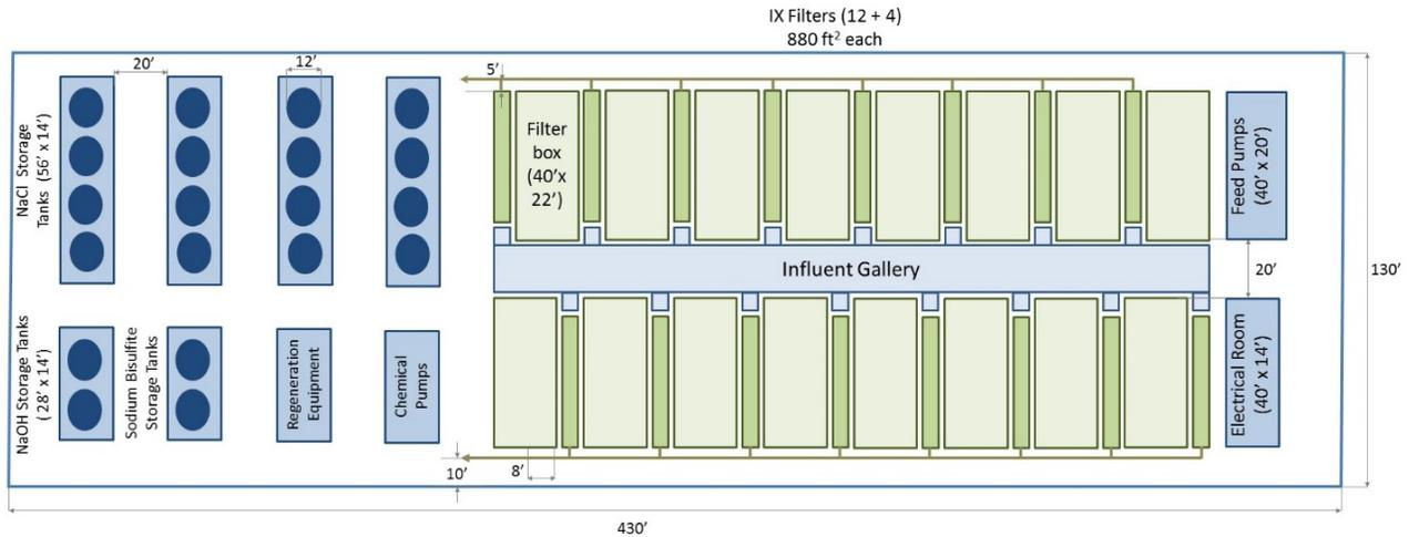
Figure 4 – Conceptual Site Layout for the Strong Base Anion IX Process
