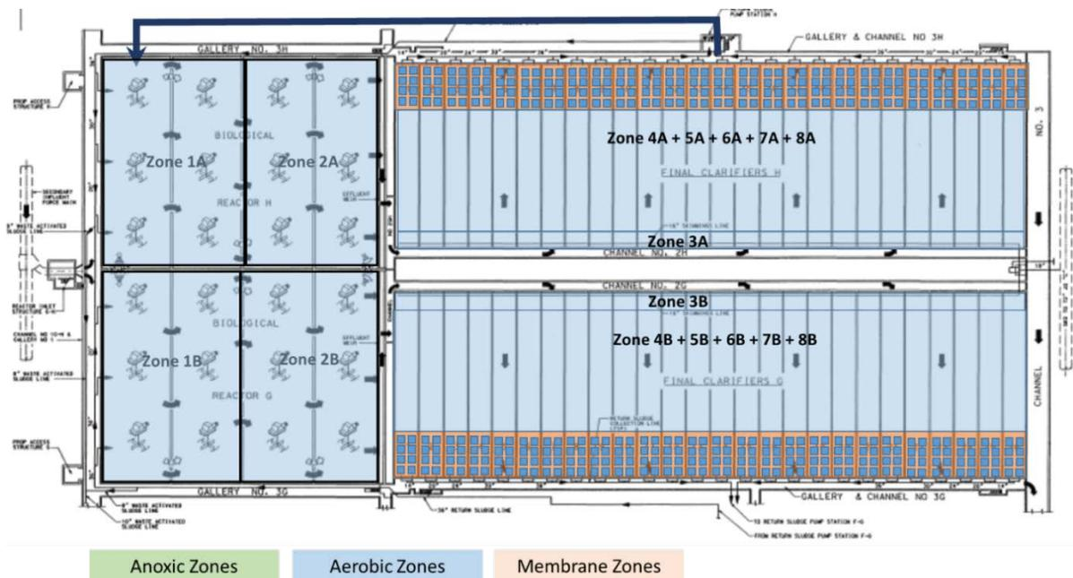
Figure 4.2 – Schematic of Secondary Facilities Retrofit to N-only Secondary MBR at JWPCP
