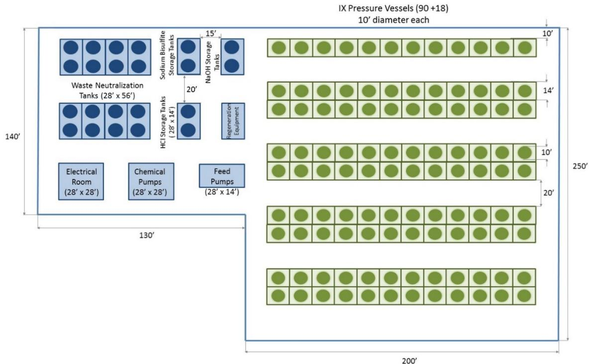
Figure 2 – Conceptual Site Layout for the Boron-selective IX Process
