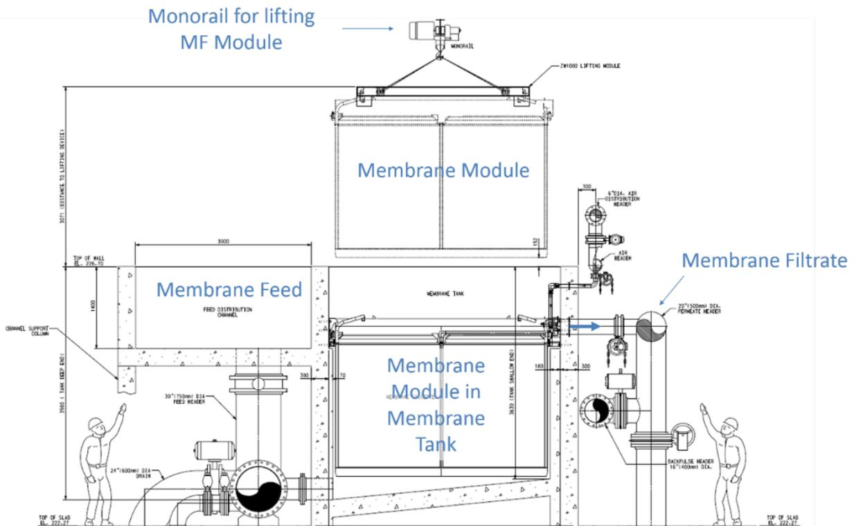
Figure 4.6 – Example Cross-section of Submerged MF System
