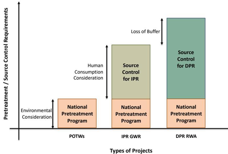
Figure 3. Growth of source control requirements with IPR and DPR
