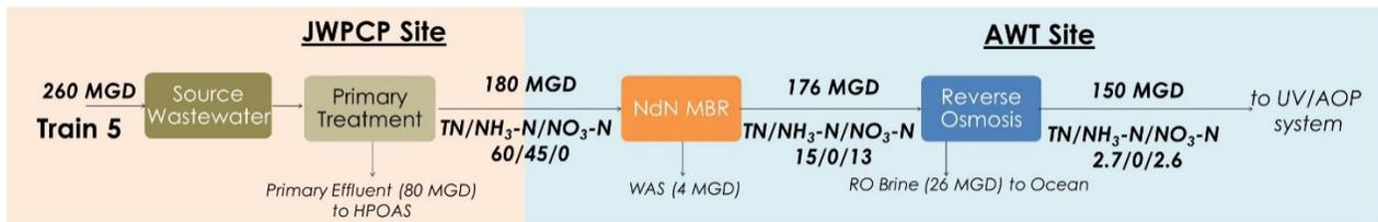
Figure 5.5 – Process Schematic for Train 5
