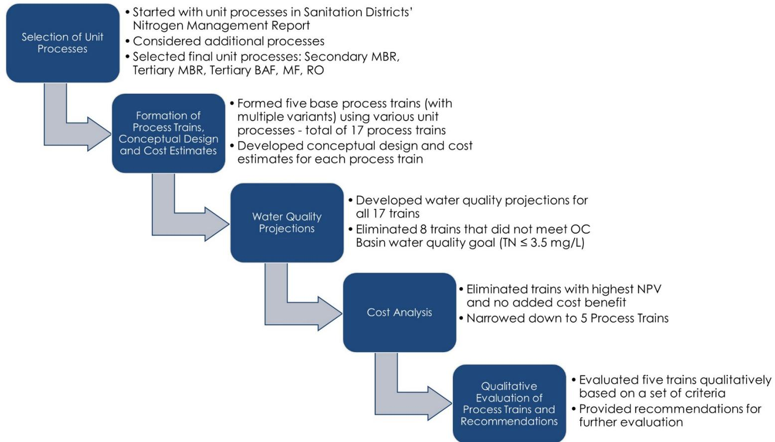
Figure 3.1 – Approach for Selection of Recommended Process Trains
