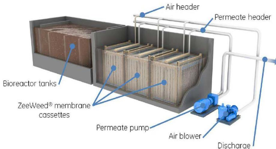
Figure 4.4 – Example Layout of GE’s ZeeWeed MBR system (Courtesy of GE)
