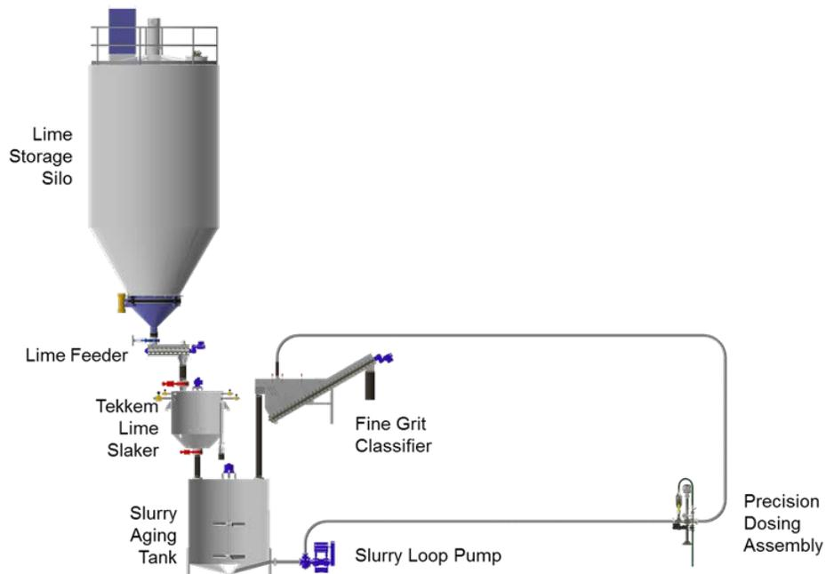
Figure 4.9 – Schematic of the Batch Lime Feeding System (Courtesy of RDP Tekkem)
