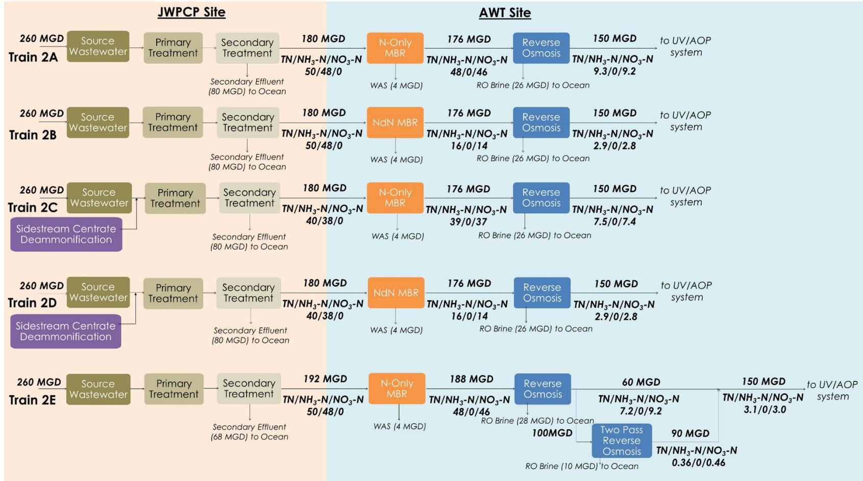
Figure 5.2 – Process Schematics of Train 2 Variants
