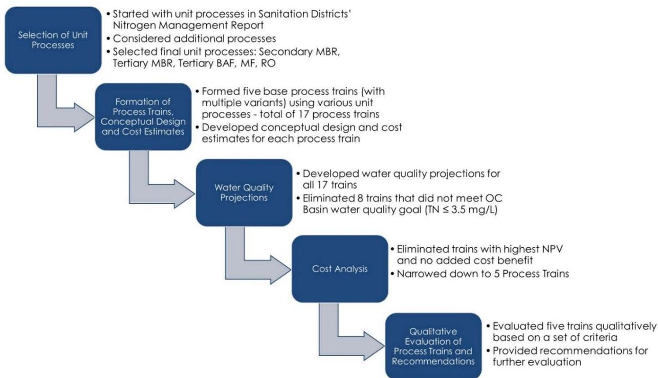
Figure 1.2 – Approach for Selection of Recommended Process Trains
