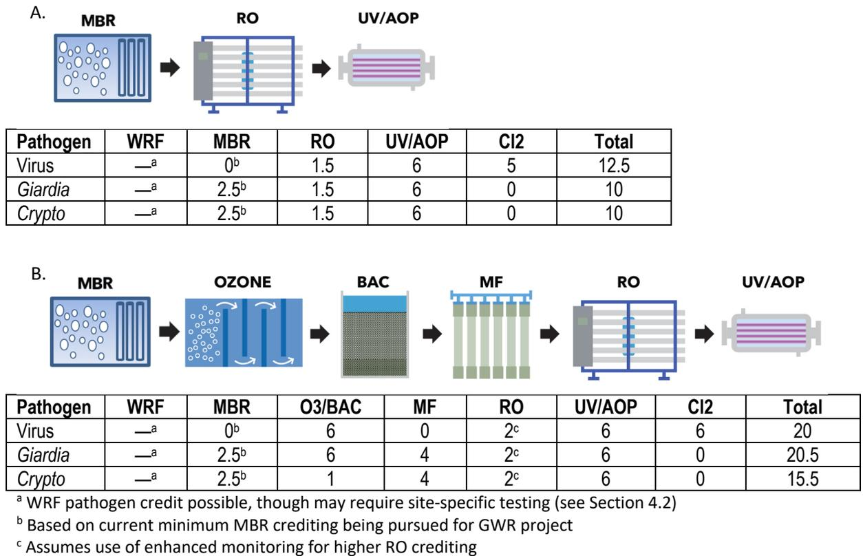
Figure 6. Pathogen log removal values of (A) the current groundwater recharge train and (B) a potential raw water augmentation train
