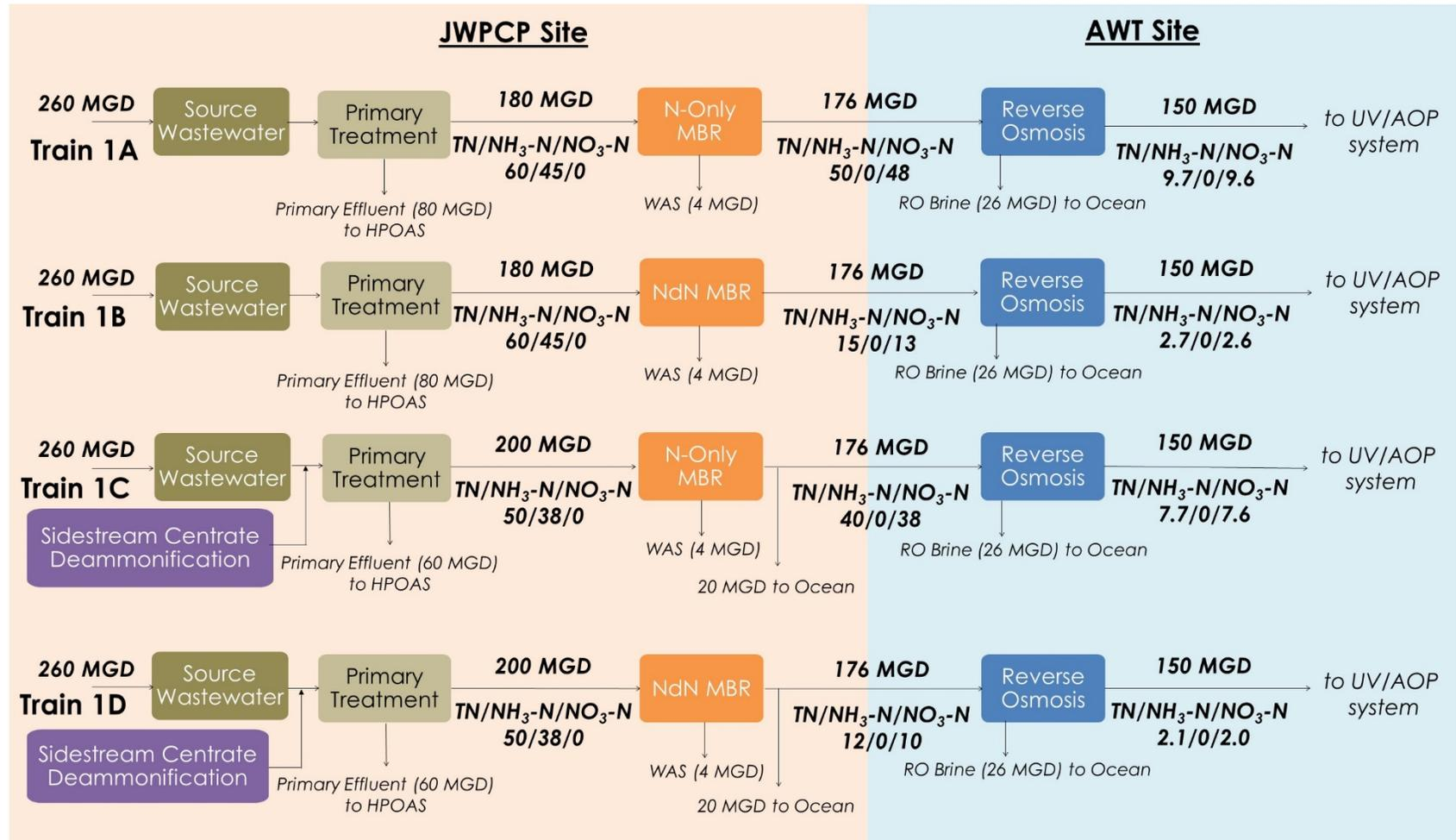
Figure 5.1 – Process Schematics for Train 1 Variants
