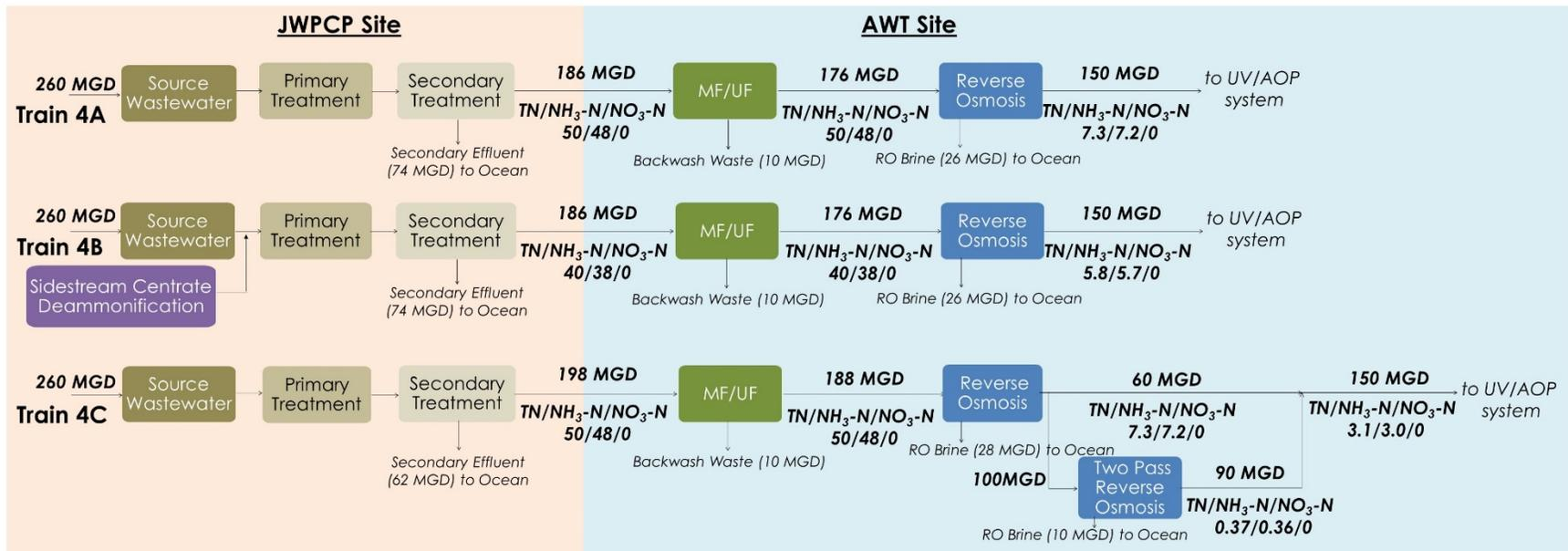
Figure 5.4 – Process Schematics for Train 4 Variants
