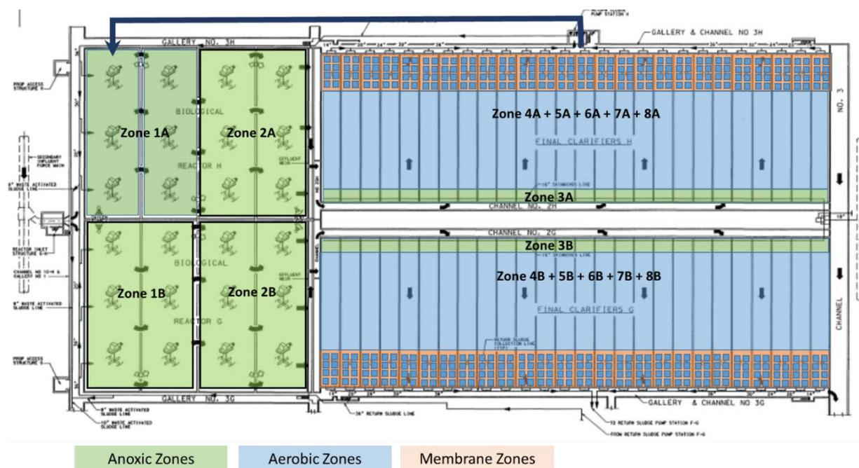
Figure 4.3 – Schematic of Secondary Facilities Retrofit to NdN Secondary MBR at JWPCP
