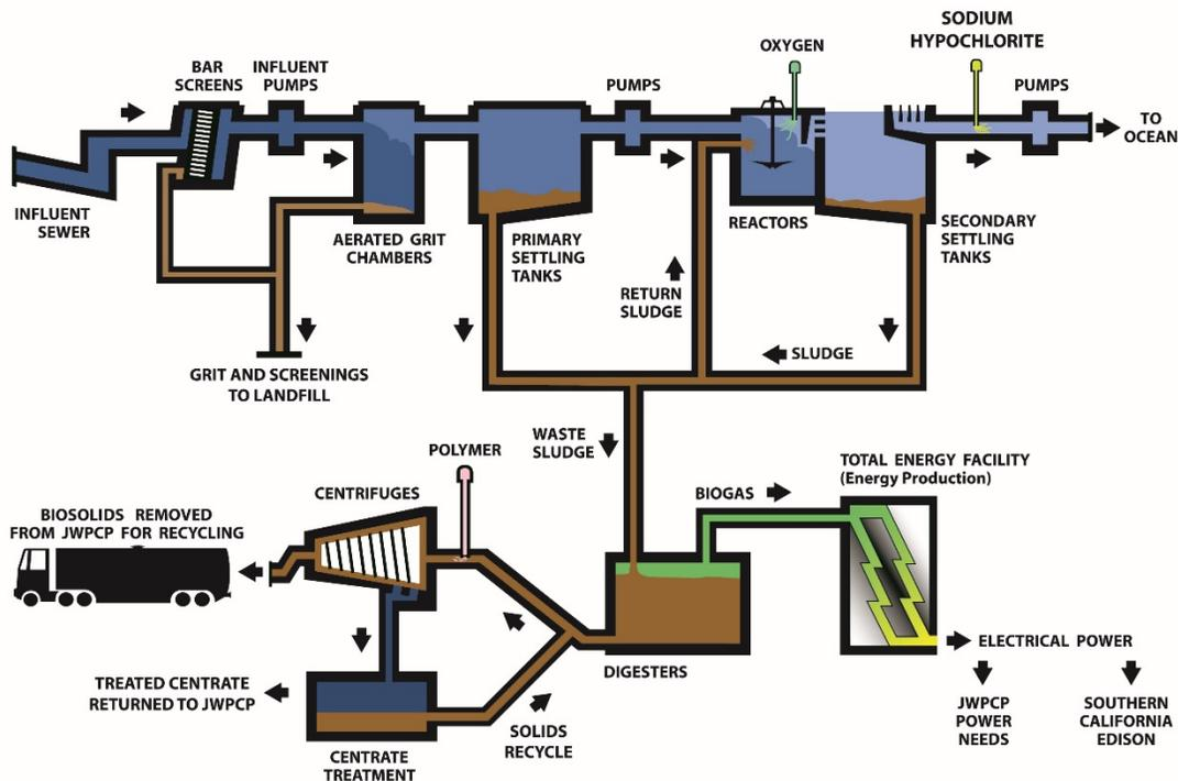
Figure 6.1 – Process Schematic of JWPCP
