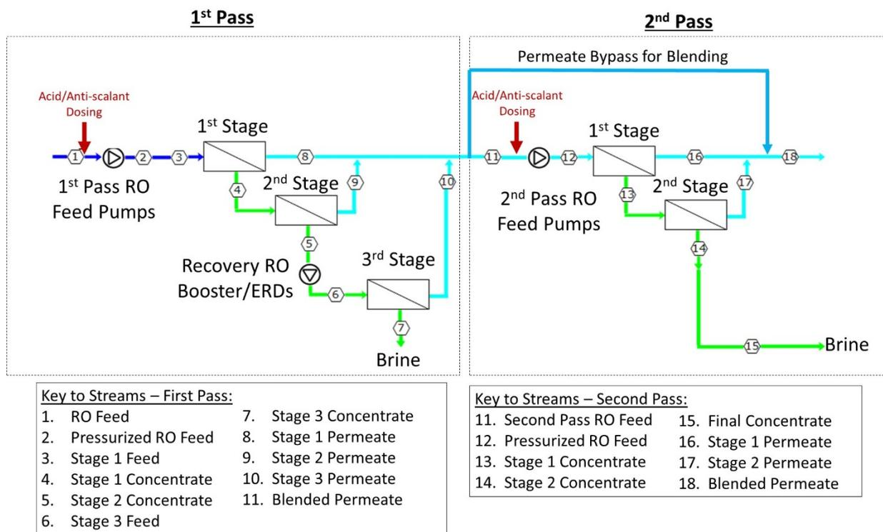
Figure 4.7 – Process Schematic of a Two Pass RO System
