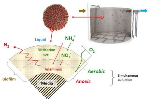
Figure 4.1 – Schematic of ANITA™ Mox Process (Courtesy of Veolia)
