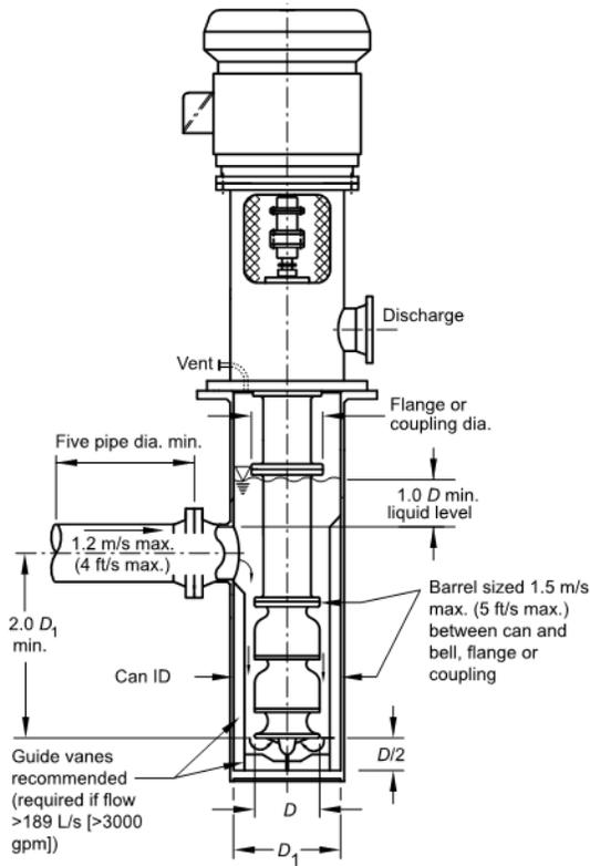
After installation of the can is complete, the mounting surface of the pumps must be level enough and the can shall be plumb to ensure that the suction bell can be centered within 3% of the suction bell diameter ( $0.03 \times D$ ).
