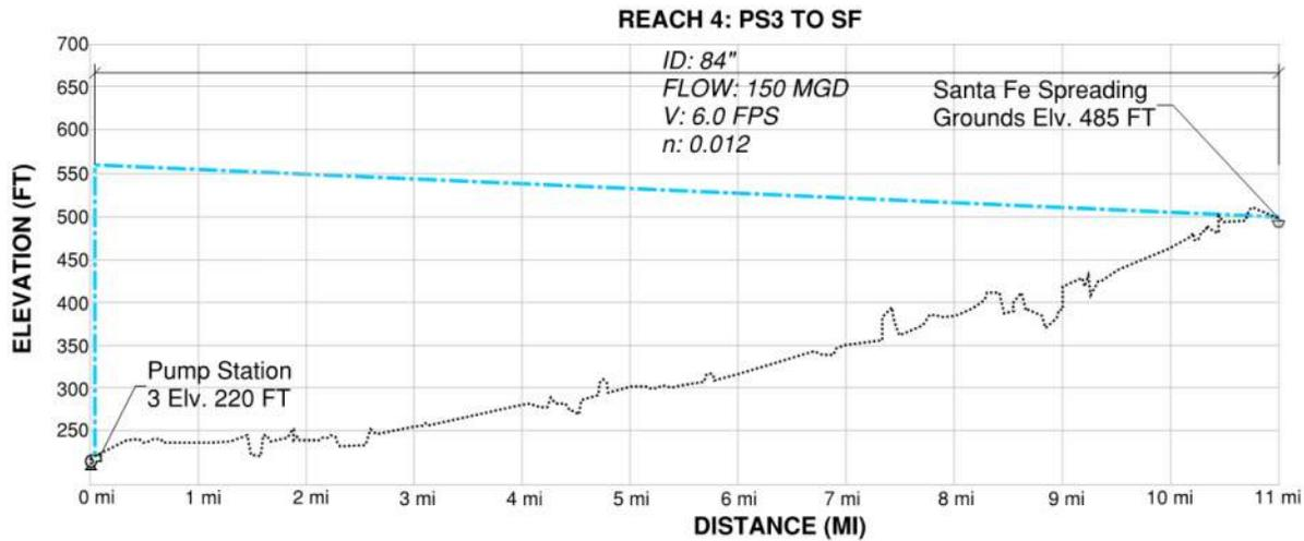
Figure 6-5 Reach 4 Hydraulic Profile (SG River Alignment)
