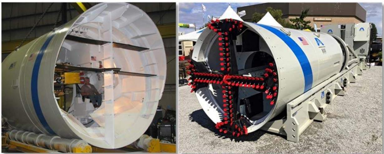
Figure 3-3 Boring/Digger Shield and Cutting Head, Akkerman
