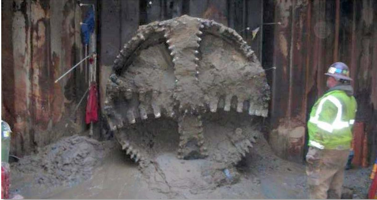
**Figure 3-6** 72-inch diameter Microtunneling Machine – East Chicago, Indiana
