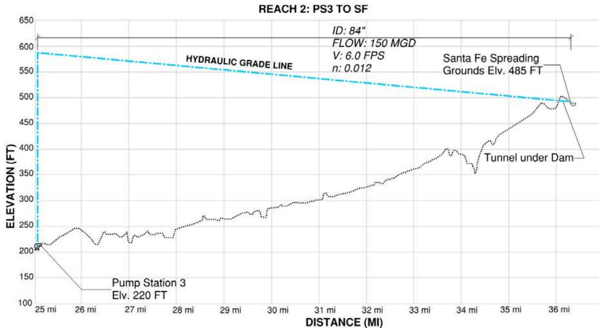
Figure 7-5 Reach 2 Hydraulic Profile (LA River Alignment)
