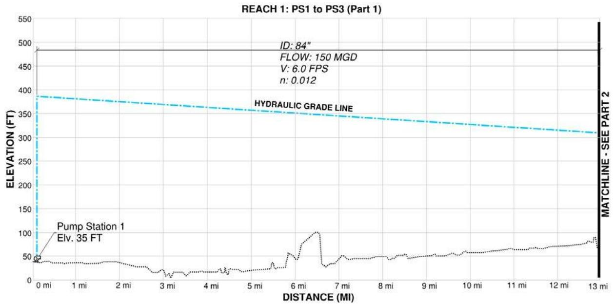
Figure 7-3 Reach 1, Part 1 Hydraulic Profile (LA River Alignment)
