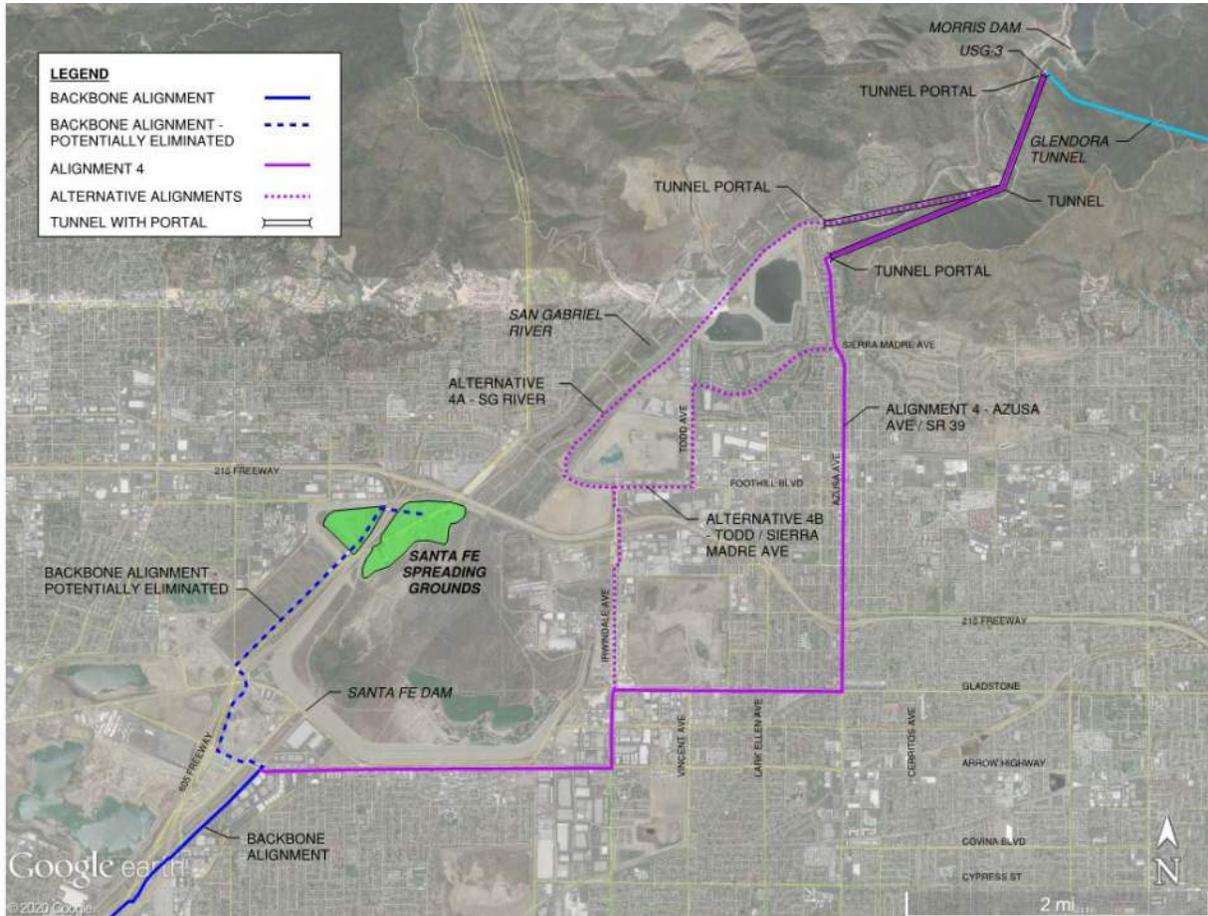
Figure 5-13 Alignment 4 – Azusa Avenue / SR 39 to Glendora Tunnel and Alternatives
