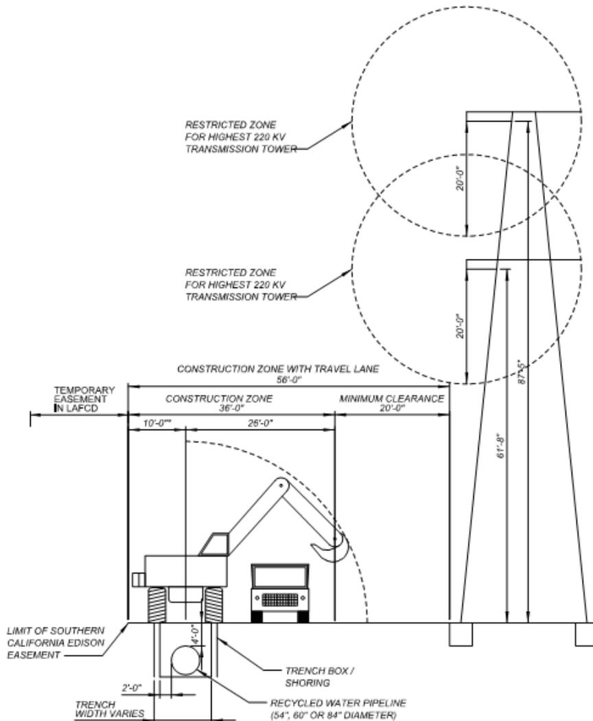
Figure 3-16 Construction Method 2 – SCE Easement (Shored Construction)
