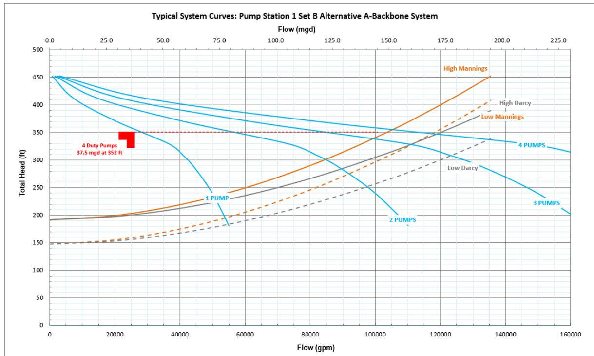
Figure 8-7 PS-1 Set B System Curves – Backbone System
