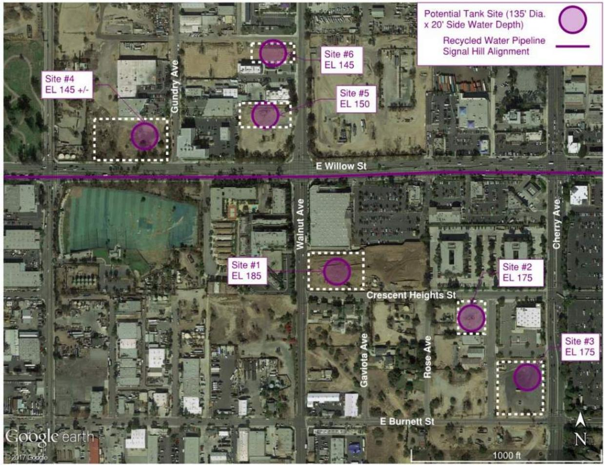
Figure 5-5 Signal Hill Tank Location Map
