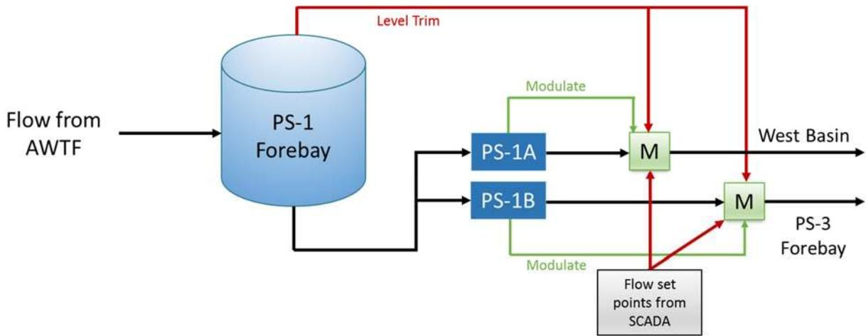
**Figure 8-3** Flow Control with Level Trim and PS-1
