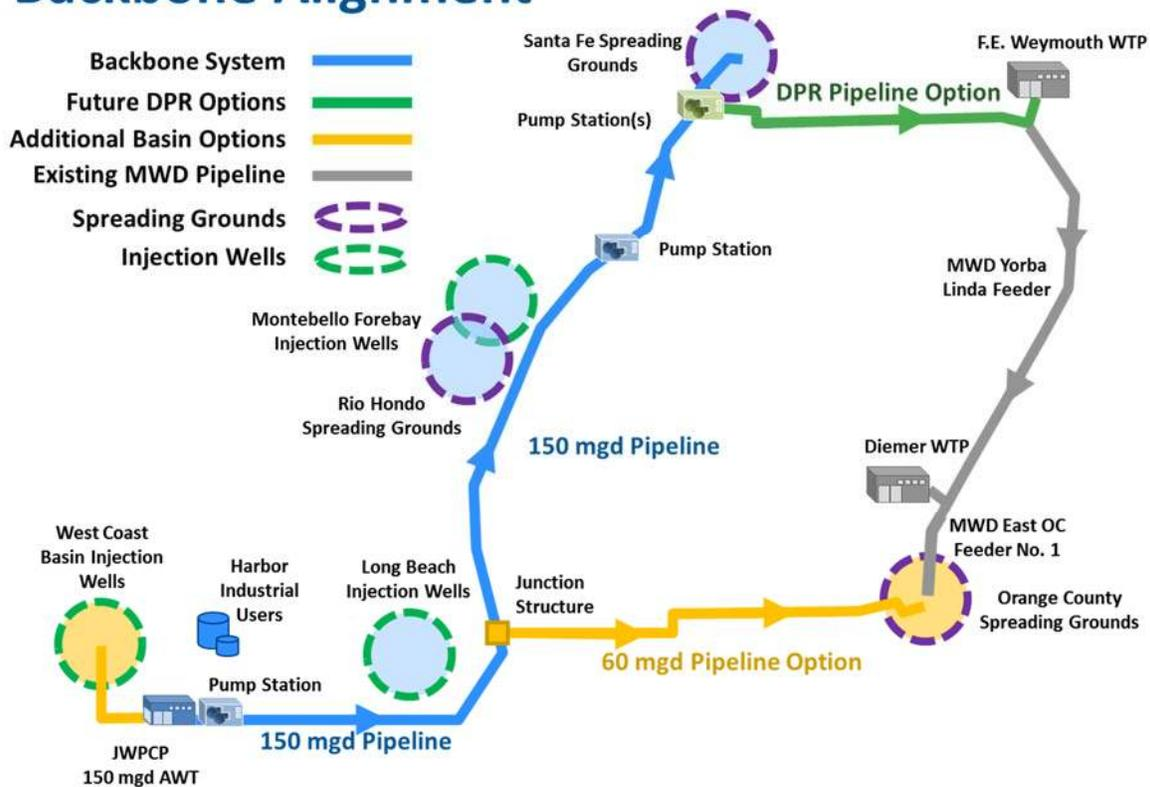
Figure 1-3 Proposed Regional Recycled Water Program Backbone System
