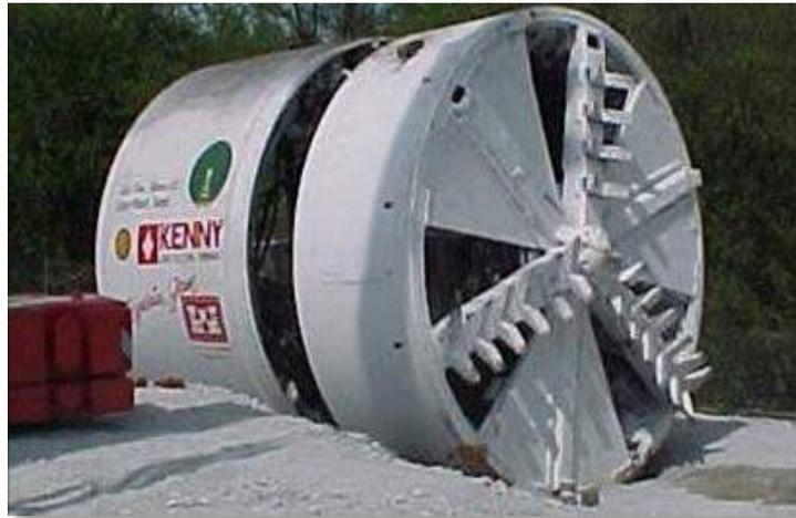
**Figure 3-7 Open Mode Shielded TBM used on Cady Marsh Stormwater Tunnel, Griffith, Indiana**
