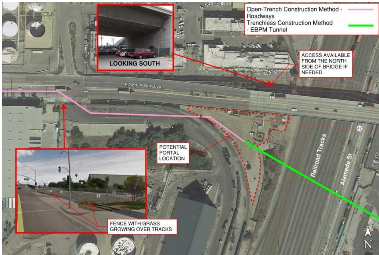
**Figure 6-8 Potential Launching Portal Site for the Alameda Corridor/Dominguez Channel Crossing (Detail Location 1)**
