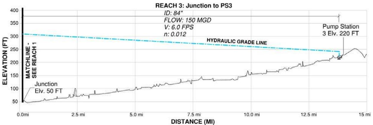
Figure 6-4 Reach 3 Hydraulic Profile (SG River Alignment)
