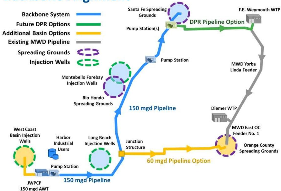
Figure 5-7 Proposed Regional Recycled Water Program Backbone System
