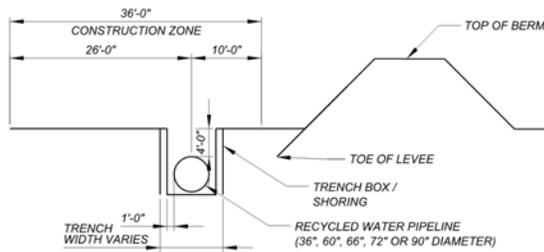
Figure 3-17 Construction Method 3A – River Bank (Shored Construction)
