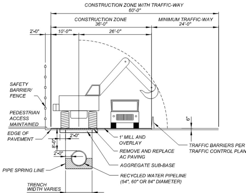
Figure 3-15 Construction Method 1 – Roadways (Shored Construction)
