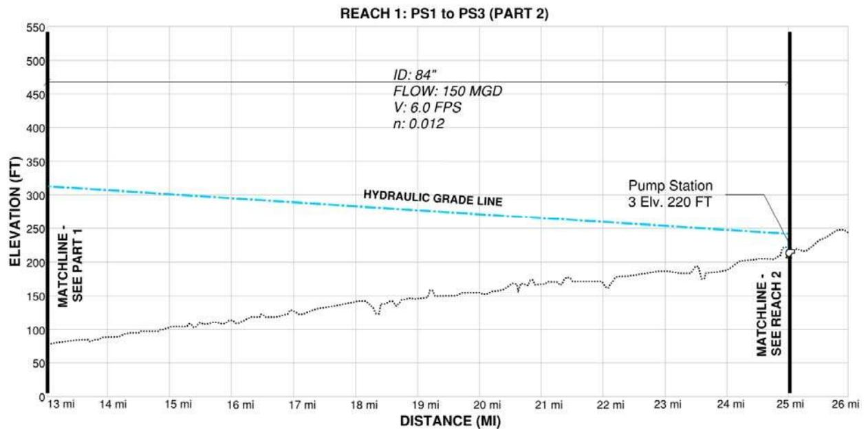
Figure 7-4 Reach 1, Part 2 Hydraulic Profile (LA River Alignment)
