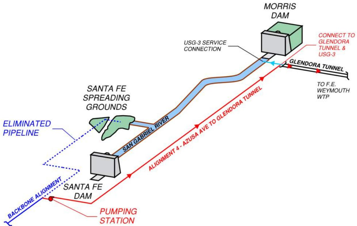
Figure 5-12 Alternative Discharge Location for Alignment 4 – Schematic View
