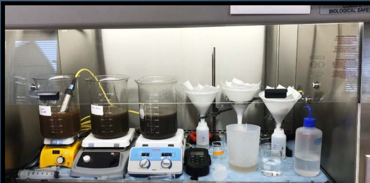
Denitrification Reactor Test Setup
