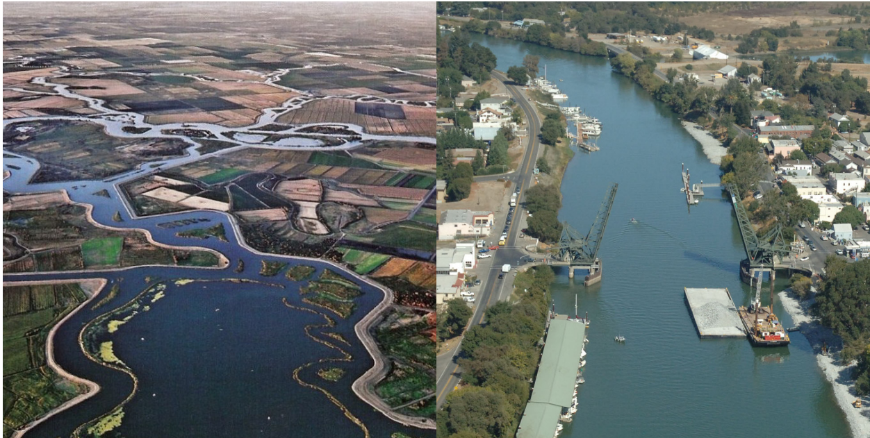
The Delta has been considered “broken” for some time. It has been altered significantly from its natural form and it is not sustainable. Land subsidence in the Delta is a direct threat to the levees (pictured right). Subsidence in the Delta has been caused by the use of land for farming and the composition of the rich peat soil. Some island areas are currently 30 feet below sea level, and extremely vulnerable to flooding. Working towards sustainable solutions in the Delta is one of Metropolitan’s Core Resources Strategies.
